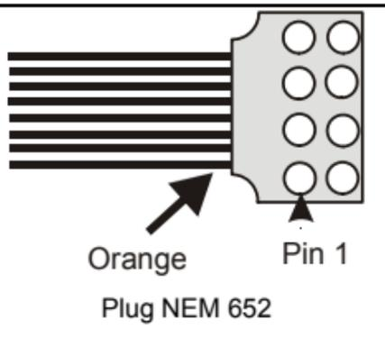
Function output D is not connected to the NEM plug.
